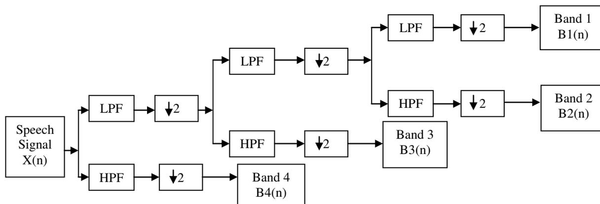
Fig 3.2 Speech signal sub band coding
