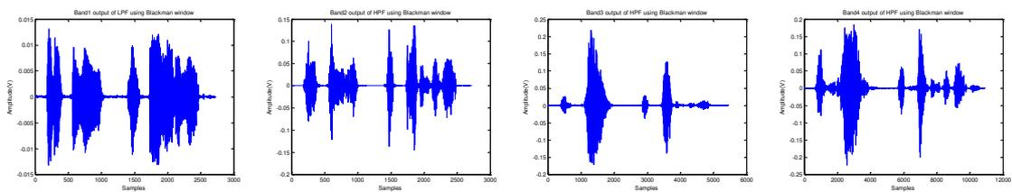
Fig 4.16 Band 1, 2, 3 and 4 outputs of Blackman window for speech signal2
