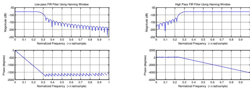
Fig 4.5 Response of LPF and HPF using Hanning Window
