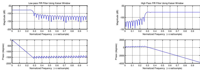
Fig 4.8 Response of LPF and HPF using Kaiser Window
