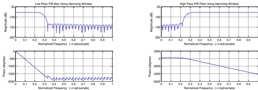
Fig 4.4 Response of LPF and HPF using Hamming Window
