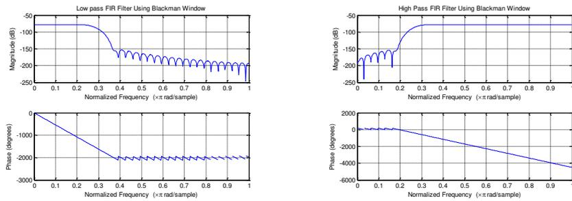
Fig 4.6 Response of LPF and HPF using Blackman Window
