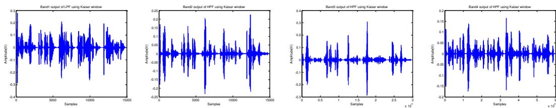
Fig 4.13 Band 1, 2, 3 and 4 outputs of Kaiser window for speech signal1
