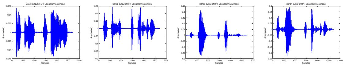
Fig 4.15 Band 1, 2, 3 and 4 outputs of Hanning window for speech signal2
