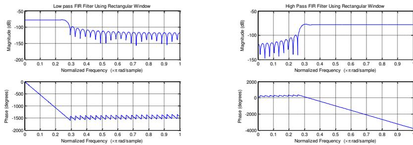
Fig 4.7 Response of LPF and HPF using Rectangular Window
