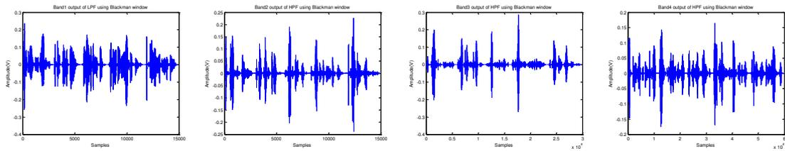
Fig 4.11 Band 1, 2, 3 and 4 outputs of Blackman window for speech signal1
