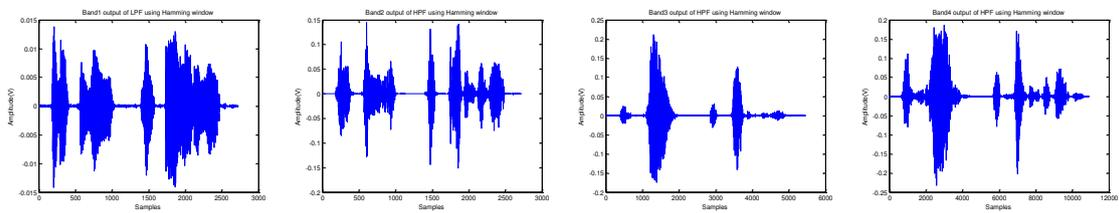
Fig 4.14 Band 1, 2, 3 and 4 outputs of Hamming window for speech signal2
